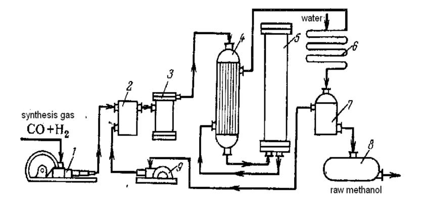
1 - compressor, 2 - mixer, 3 – filter, 4 - heat exchanger, 5
